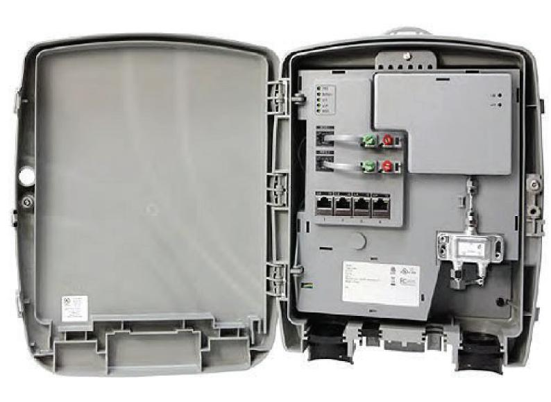
Design of Optical Network Terminal(ONT) for Gigabit Passive Optical Network(GPON)
